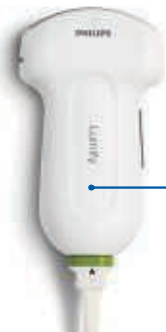
Lumify C5-2 broadband curved array transducer
